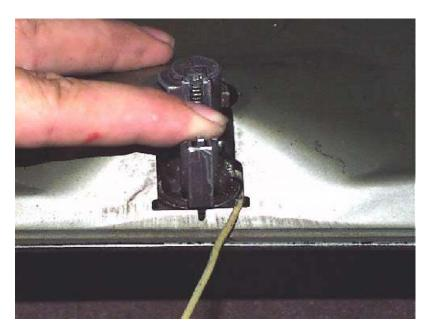
5) The lock cylinder should start to pop out a little. Keep the latch pressed.
