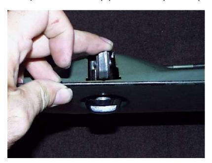
6) Keep wiggling the tool, and the cylinder should come the rest of the way out. What you are trying to accomplish is to depress each tumbler (not sure if thats the right terminology), so that the cylinder can come out past that point:
